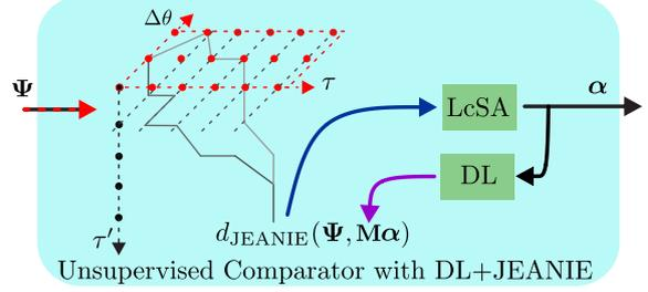
Fig. 8: Unsupervised FSAR uses the JEANIE measure as a distance between feature map  $\Psi$  of a sequence and its dictionary-based reconstruction  $\mathbf{M}\alpha$ . LcSA performs feature coding to obtain dictionary-coded  $\alpha$ . DL learns the dictionary  $\mathbf{M}$ .
