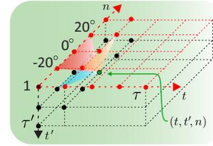
Fig. 6: JEANIE (1-max shift). We loop over all points. At  $(t, t', n)$  (green point) we add its base distance to the minimum of accumulated distances at  $(t, t'-1, n-1)$ ,  $(t, t'-1, n)$ ,  $(t, t'-1, n+1)$  (orange plane),  $(t-1, t'-1, n-1)$ ,  $(t-1, t'-1, n)$ ,  $(t-1, t'-1, n+1)$  (red plane) and  $(t-1, t', n-1)$ ,  $(t-1, t', n)$ ,  $(t-1, t', n+1)$  (blue plane).
